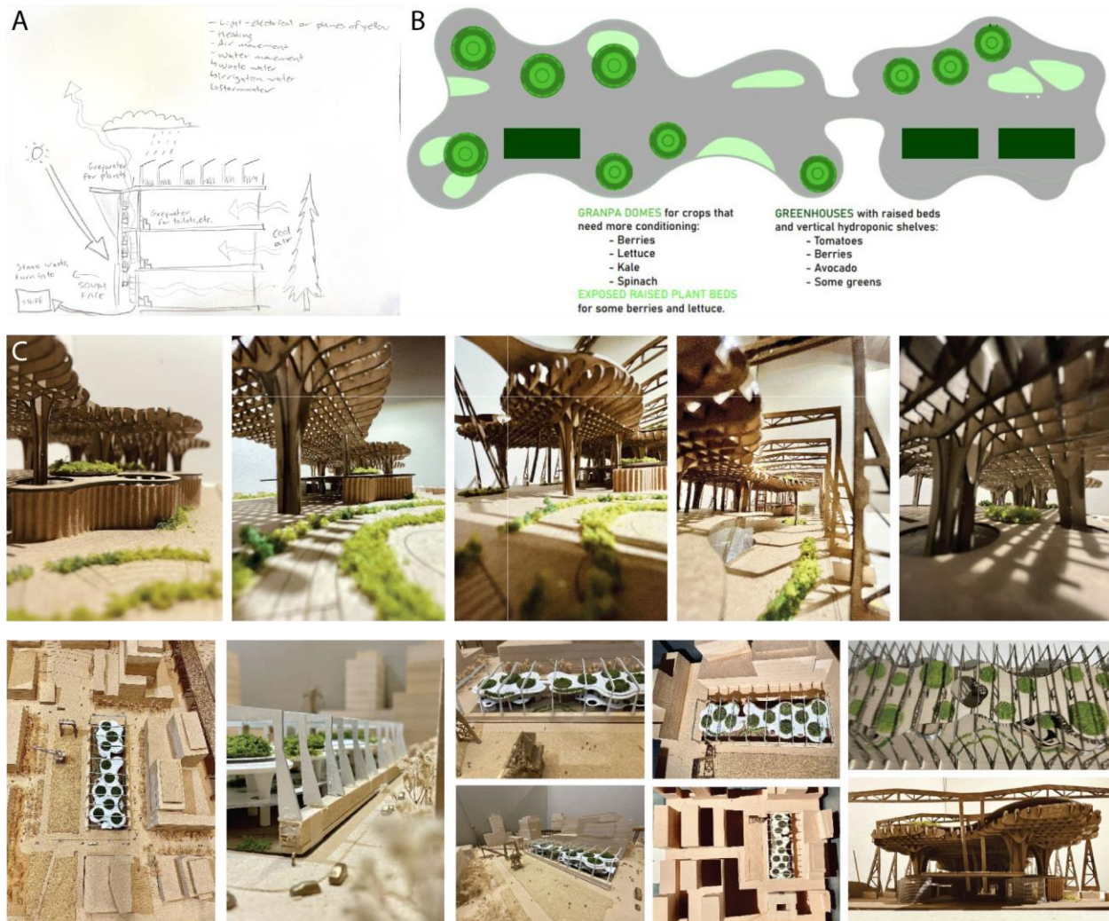
Figure 3. Team 2 design showing A) early ideation sketches, B) final organization of agricultural program using inflatable greenhouse structures known as Granpa Domes, and C) vignettes of final models at 1/16" = 1'0" (brown chipboard) and 1/32" = 1'0" (white museum-board).
